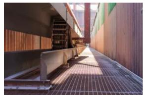
Recently, the motorised cable drums on the cranes for loading and unloading ships were exchanged and equipped with e-chains from igus. (Source: igus GmbH)
