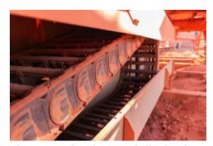
The stress by dust and dirt is also very high in the stockyard. An e-chain with external stop-dogs is used here, whereby there is less accumulation of dust here. (Source: igus GmbH)
