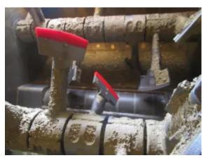
The three-dimensional mixing concept results in an intensive exchange of materials, and shorter mixing cycles with reduced energy consumption.
