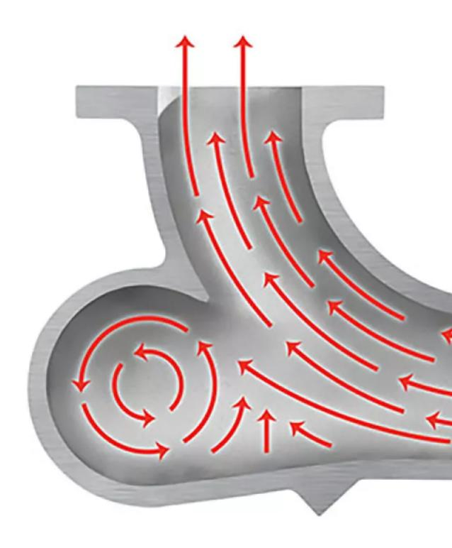
The teardrop-shaped vortex chamber of the short radius elbow protrudes partially began a sphere of material-in-air to rotate in the same direction as the air stream, gently debend.
