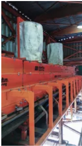
The skirtboard cover is shown with two dust bags.
