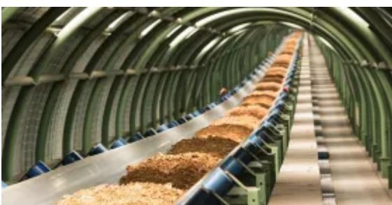
View of the enclosed conveyor flight in the area of the bridge.
