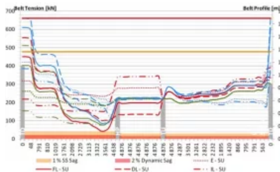
Fig. 11: Tension Distribution during Various stationary and non stationary cases
