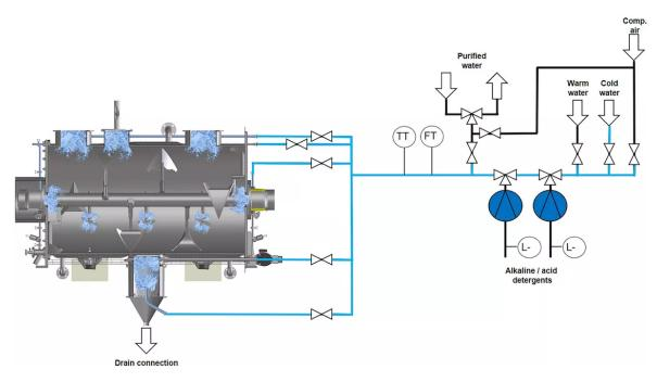
Schematic diagram of a WIP system with typical rinsing points on a horizontal Ploughshare Mixer. (Source: Lödige)
