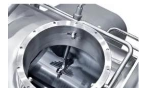
Example of a feeding socket with fixed cleaning nozzles and flushing supply (Source: Lödige)
