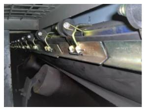
Conveyor skirting maintains a dust seal between the chute structure and the conveyor belt. (Pictures: @Dyna Engineering)
