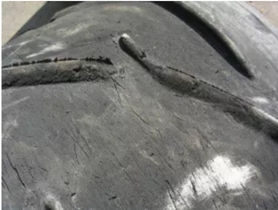
Fig. 2: Chevrons as high as 25mm or 32mm can wear almost completely flat in a remarkably short time.
