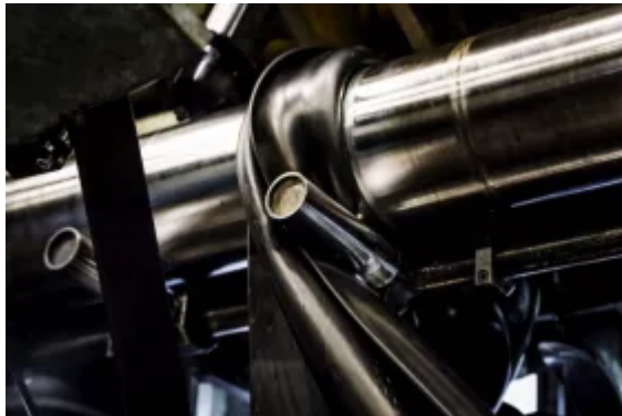
Fig. 3: A 'single structure' chevron belt needs a highly specialised rubber.
