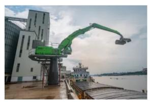
The 12-meter banana boom and 5-meter pylon provide easy access to deep cargo holds and a clear view of the jetty and vessel.
