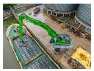
The machine unloads around 250 tons of raw materials per hour with four cycles per minute, ensuring a steady, rapid supply to the mill. (Pictures: ©SENNEBOGEN)
