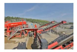
CDE introduced the ability to further remove some of the 0.250mm material after the CFCU which can be either discharged away from the 0-2mm washed sand or proportionally reintroduced to it to nurture the 0-2mm grading according to the requirement.
