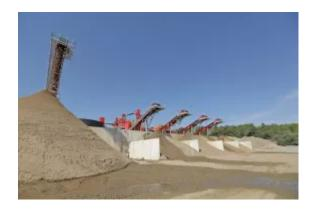
The plant allows Swerock to produce 7 products; the 0-2mm used in concrete production,2 additional sand fractions in 0-0.250mm and 2-4mm, 4 aggregate fractions in 4-16mm, 16-32mm, 32-100mm and +100mm used for a variety of construction and infrastructure projects.
