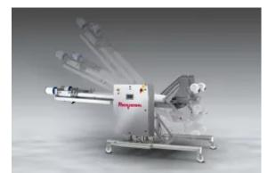
Twin BEV-CON<sup>™</sup> Flexible Screw Conveyor system with dual hoppers on a mobile base transfers difficult-to-convey materials at multiple plant locations, simultaneously or separately, and can be rolled to a washdown station for sanitising. (Picture: ©Flexicon Europe Ltd.) Each 113-liter hopper is equipped with grates capable of supporting a 115 kg bag of material, level sensors, and mechanical agitator assemblies to promote flow into the conveyor inlets.
