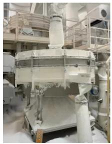
Before the switch to BFM® fitting, the customer experienced a lot of dust and material loss from their sifters. (Pictures: ©BFM® fitting)
