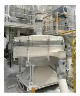
The switch to BFM® fitting stopped the leakage of the fine powder.
