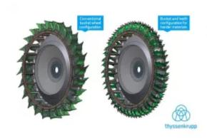
At bauma 2016 thyssenkrupp will also be presenting a new generation of compact bucket wheel excavators: the "Barracuda" and the "Mine Shark". Both machines can be used to mine hard materials with compressive strengths of up to 50 MPa. A model of the "Barracuda" can be seen at the thyssenkrupp Industrial Solutions booth.
