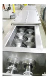
All four of the mixers include spray bars allowing water to be added to the dry salt; the mixers also each feature hinged stainless steel covers enabling the machines to be easily inspected.
