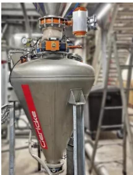
Gericke pneumatic dense phase conveying system for cocoa powder.
