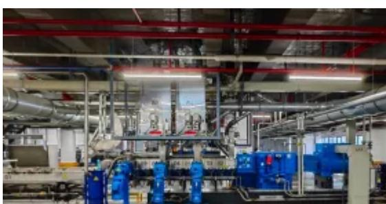
Chuanghe has acquired four of Coperion's high-performance ZSK Mc<sup>18</sup> twin screw extruders. (*Photo: Chuanghe new material technology, PR China*)
