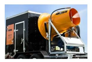
Each liquid-bearing component is insulated, heat traced or both, ensuring effective operation during cold weather.
