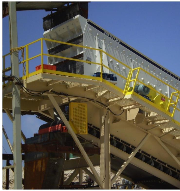
Haver & Boecker offers the versatile two-bearing Tyler T-Class vibrating screen for a wide range of material types and sizes.
