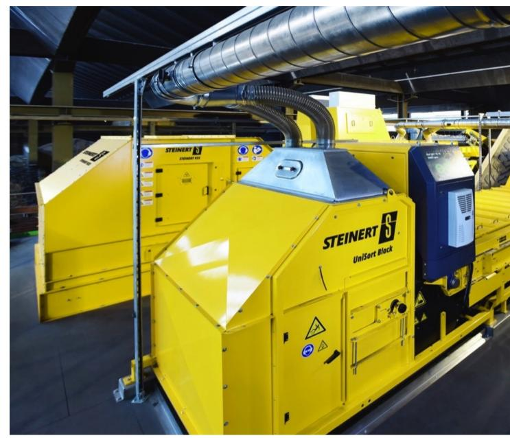
A compact system for flexible tasks: the combination sorting system Steinert KSS (back) and UniSort Black (front).
