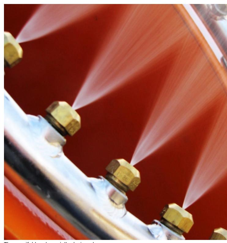
The manifold and specially-designed nozzles atomize the water supply for maximum particle attraction.
