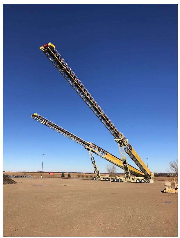
The 210 ft (64 m) long TeleStacker® Conveyor is shown next to a shorter model...a 170 ft (52 m).
