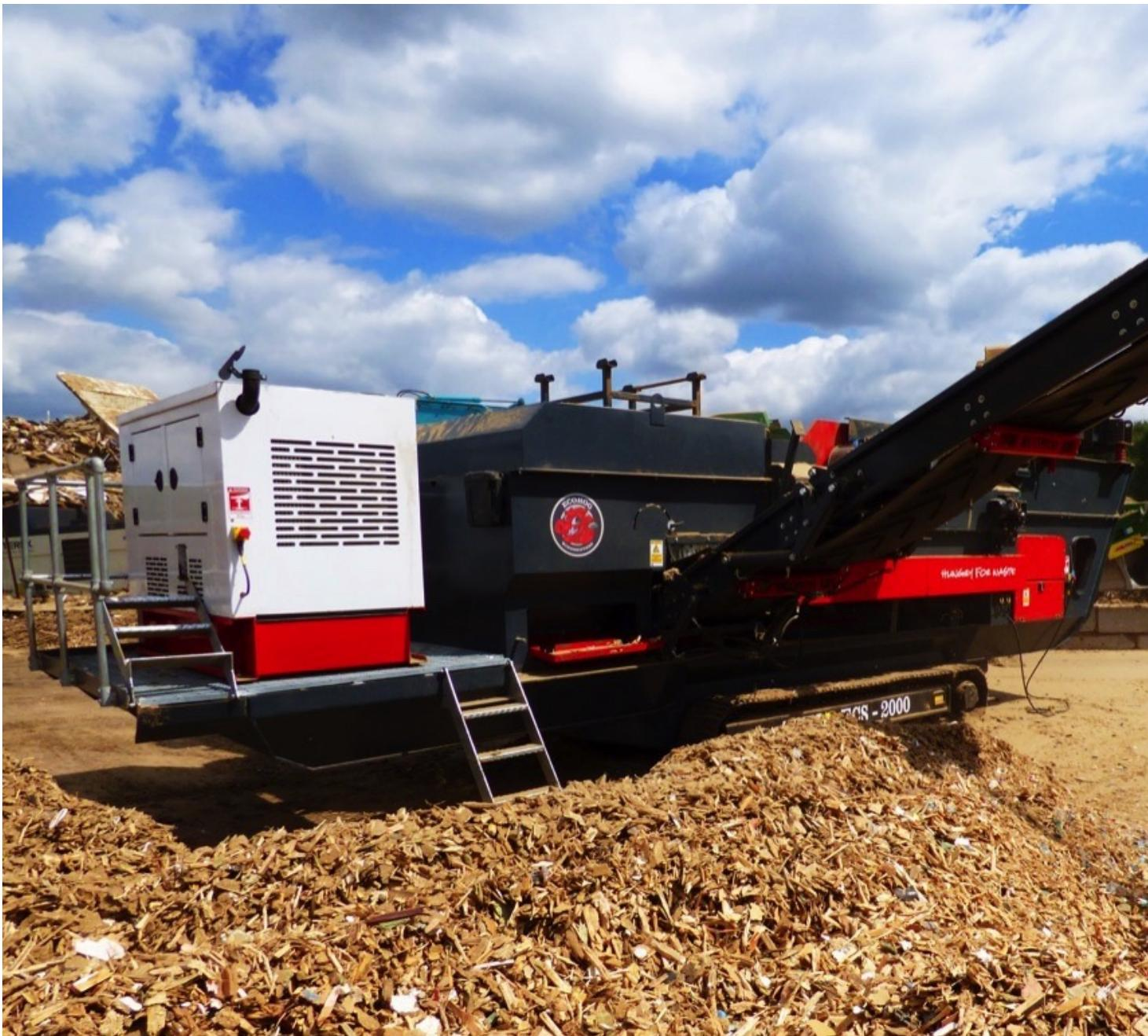
The HogMag unit incorporates an Eriez magnetic drum separator in order to remove ferrous metals such as iron and steel from all waste streams and prevent potential damage to downstream equipment.
