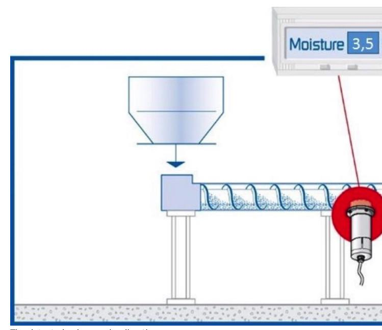
The detected value can be directly used to adapt the speed of the conveyor belt in the drying oven.
