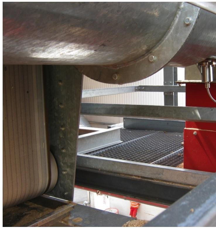
The moisture is measured while the material is transported by a screw conveyor from the oven to the storage silo.
