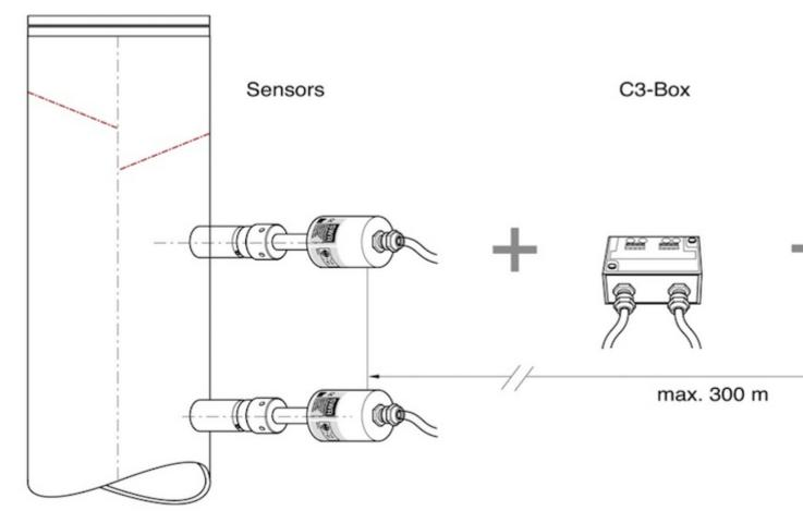
The sensors are connected to an evaluation unit via a C3 box.
