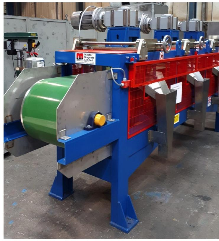
Magnetic Disc Separator in the final stages of manufacture.
