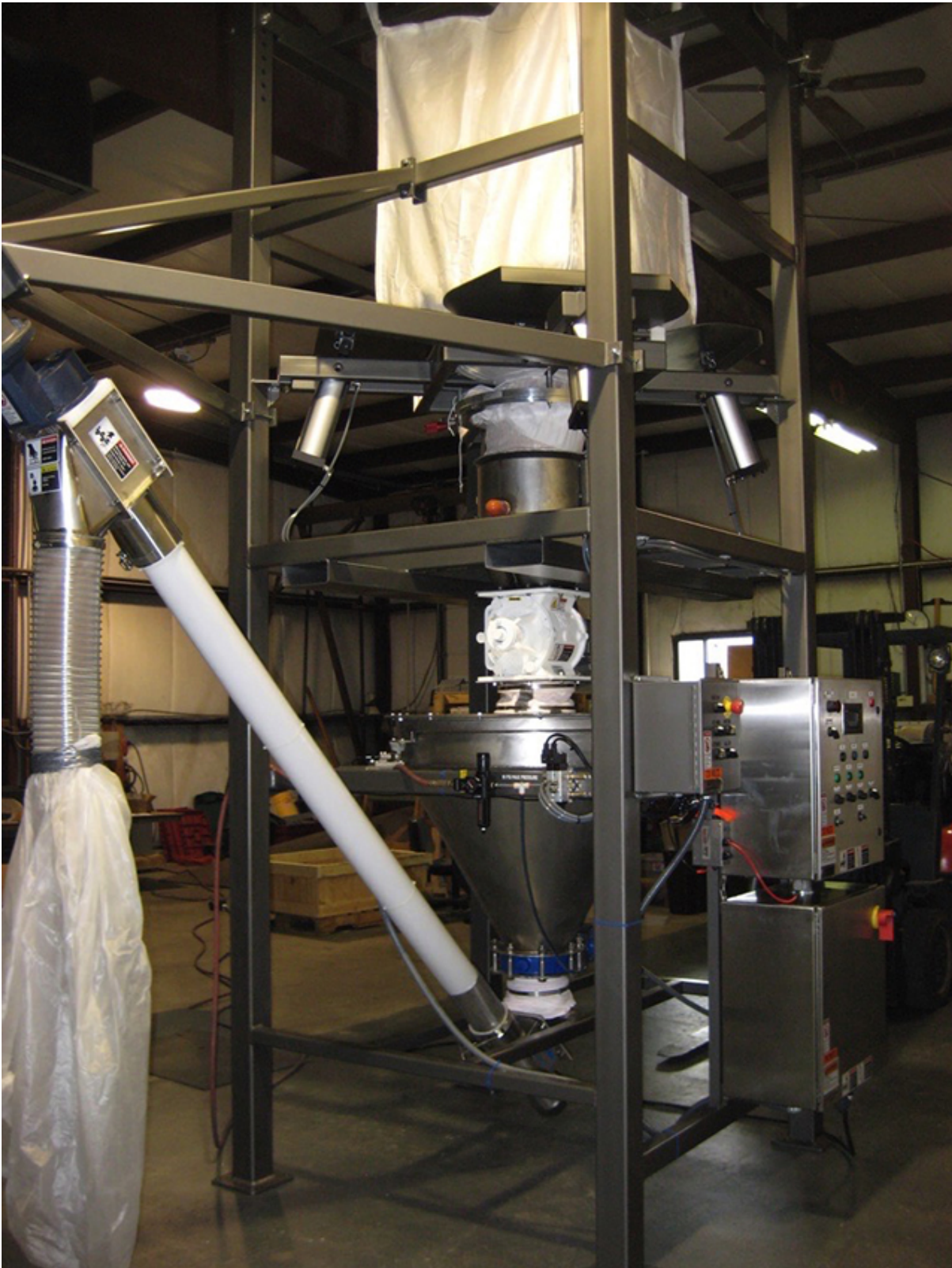
Fig. 1: Bulk bag unloading system with batch weighing, discharge and controls.
