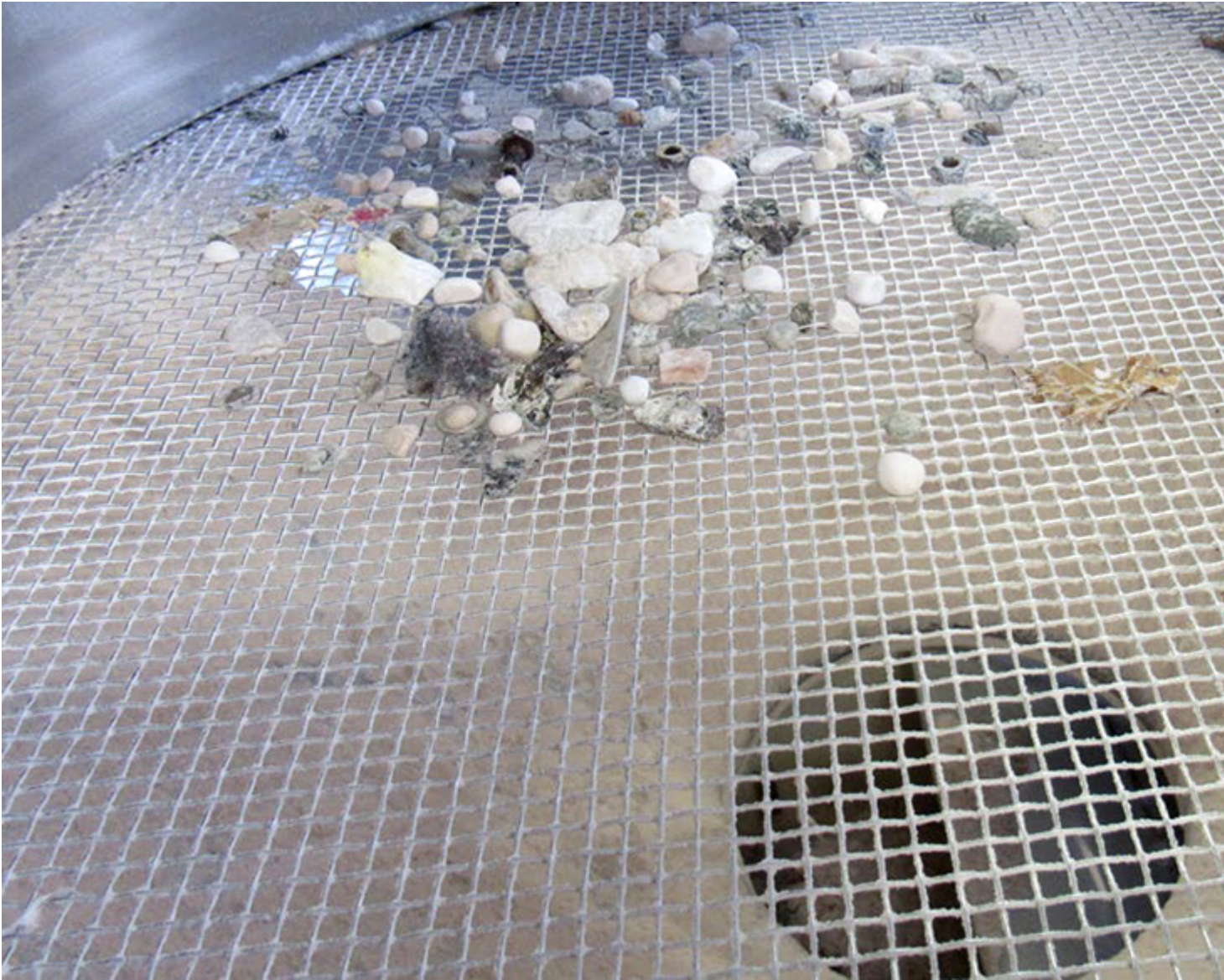
Figure 3. The Russell Compact Sieve ® removes contamination from aluminium hydrate powders, protecting chemical processing equipment.
