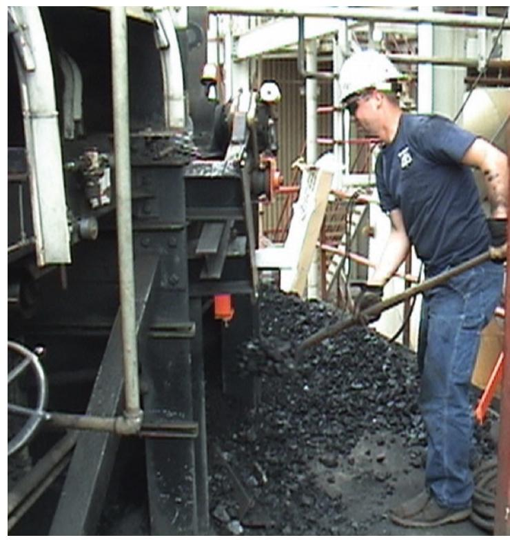
Cleaning up spillage exposes workers to a potential hazard area from the moving conveyor.
