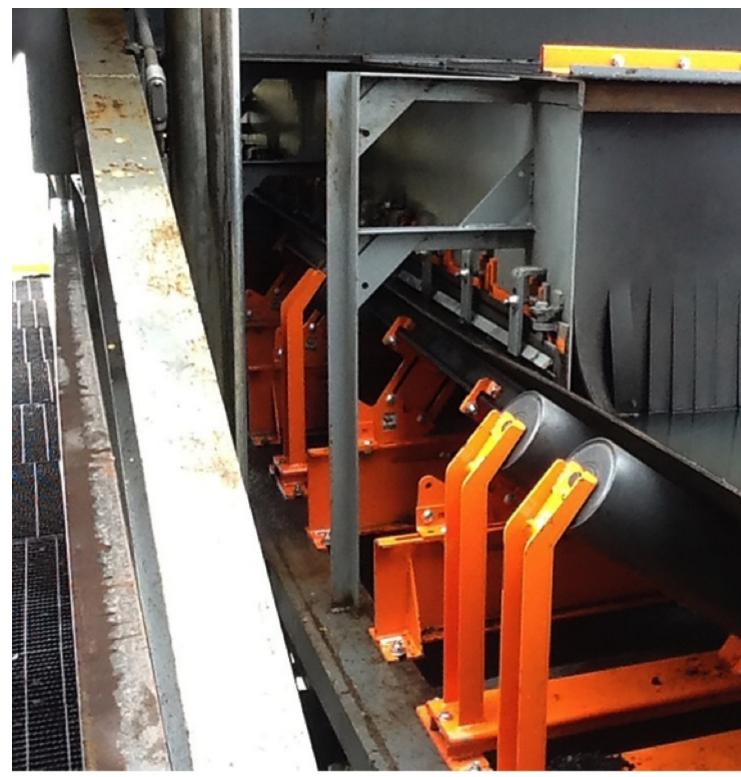
An effective transfer point requires the belt's line of travel to be stabilized and supported.
