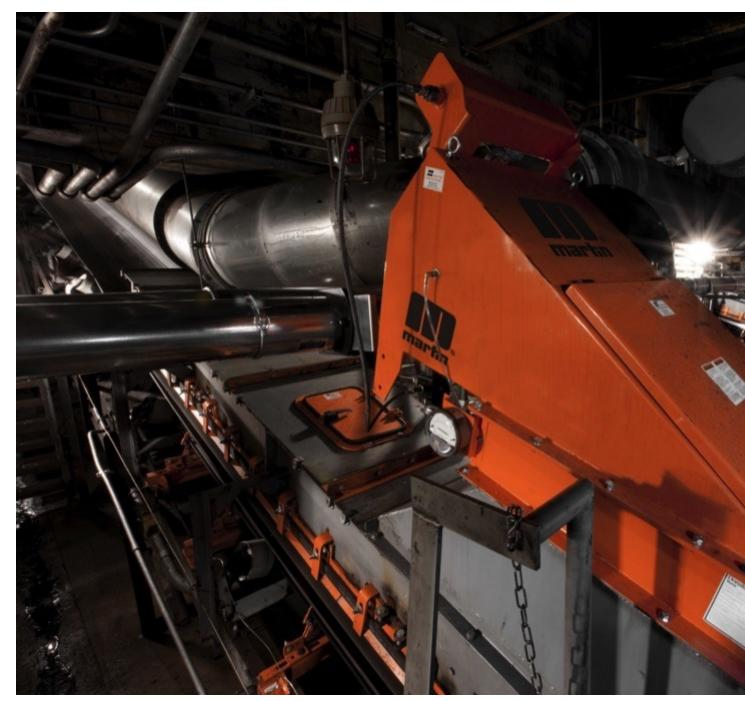
An integrated air cleaner is a small, independently-operating unit placed at the dust generation point
