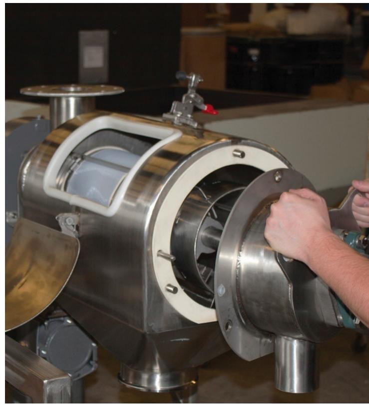
A shaft-end housing with discharge port and exterior bearing can be removed with screw knobs for access to change, inspect or clean the screen and paddles.
