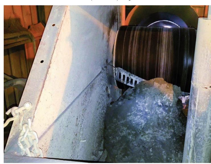
Mounted diagonally, commonly at a  $17^{\circ}$  angle, the Cleanscrape spans the entire belt profile.
