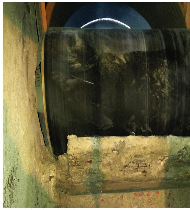
The previous blade heaped up and encrusted material, degrading cleaning performance.
