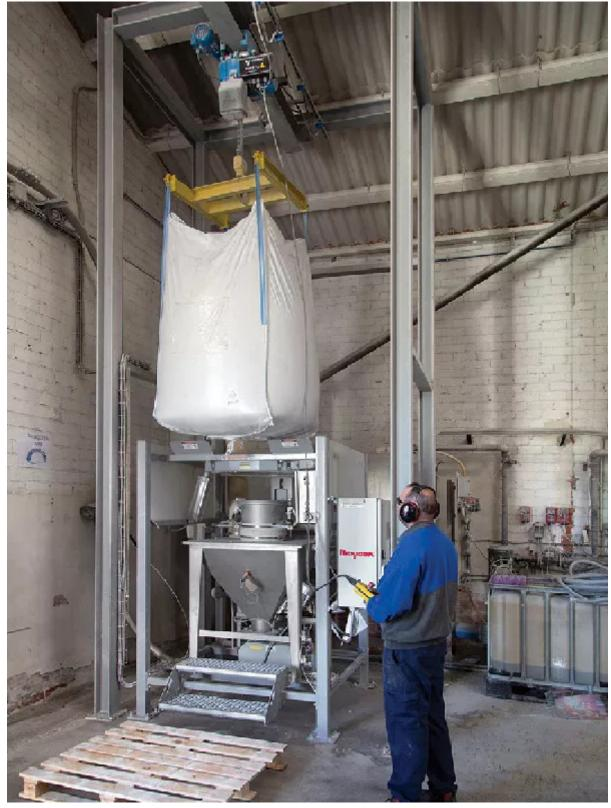
The cantilevered hoist and trolley position the bag for discharge into the 226 I hopper and through a rotary valve into the pneumatic line.
