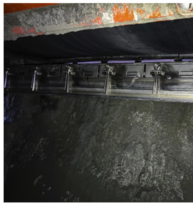
The unique stainless steel design incorporates a matrix of spring-loaded carbide tips.
