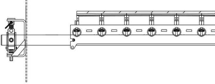
The matrix of carbide tips is tensioned lightly to prevent damage to the belt or splices.
