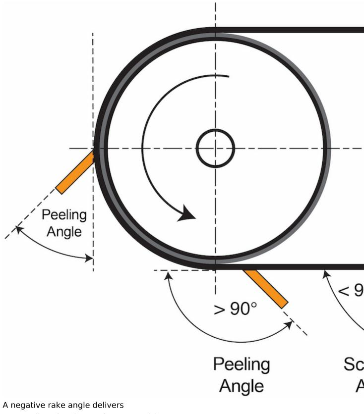
A negative rake angle delivers outstanding cleaning performance with low belt pressure.
