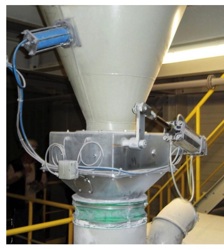
Where the bulk material flow is disrupted or irregular, putting the silo outlet (hopper) into vibration often is the only applicable solution. This has to be done carefully in order to avoid damage to the silo hopper and can be achieved by using pneumatic knockers, e.g. from <u>Singold Gerätetechnik</u>.The pneumatic knocker is used for bulk goods with material flow problems such as bridge, siphon and residue formations, when high speed shakers and vibrators with soft sine-
