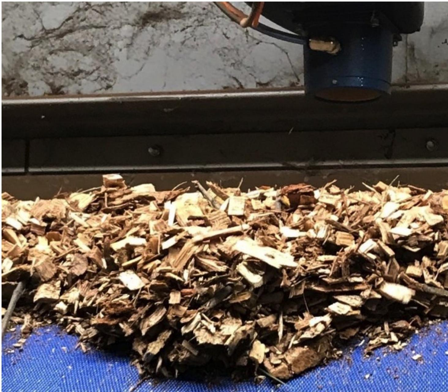
Near-Infrared moisture measurement offers clear advantages over the traditional methods. (Picture: @MoistTech)
