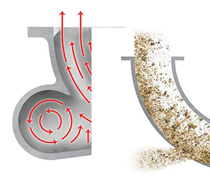
The teardrop-shaped vortex chamber of the short radius elbow protrudes partially beyond the 90-degree flow path, causing a sphere of material-inair to rotate in the same direction as the air stream, gently deflecting incoming material around the bend.
