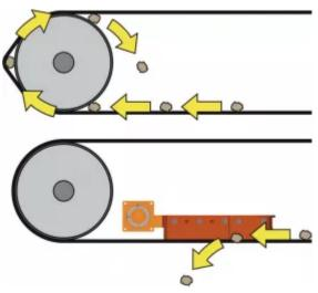
The V-Plow prevents material entrapment between the belt and tail pulley from becoming a repeating phenomenon.
