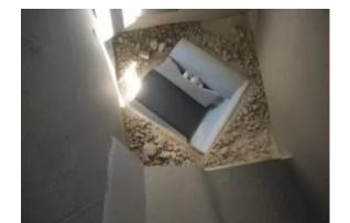
A rock box acts like a shelf, catching and distributing falling material onto the impact cradle.
