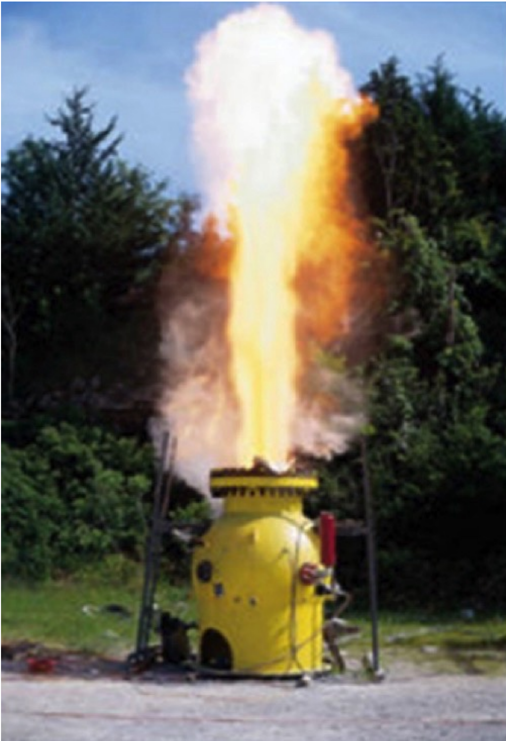
Fig. 6: explosion test without and with flameless vent.
