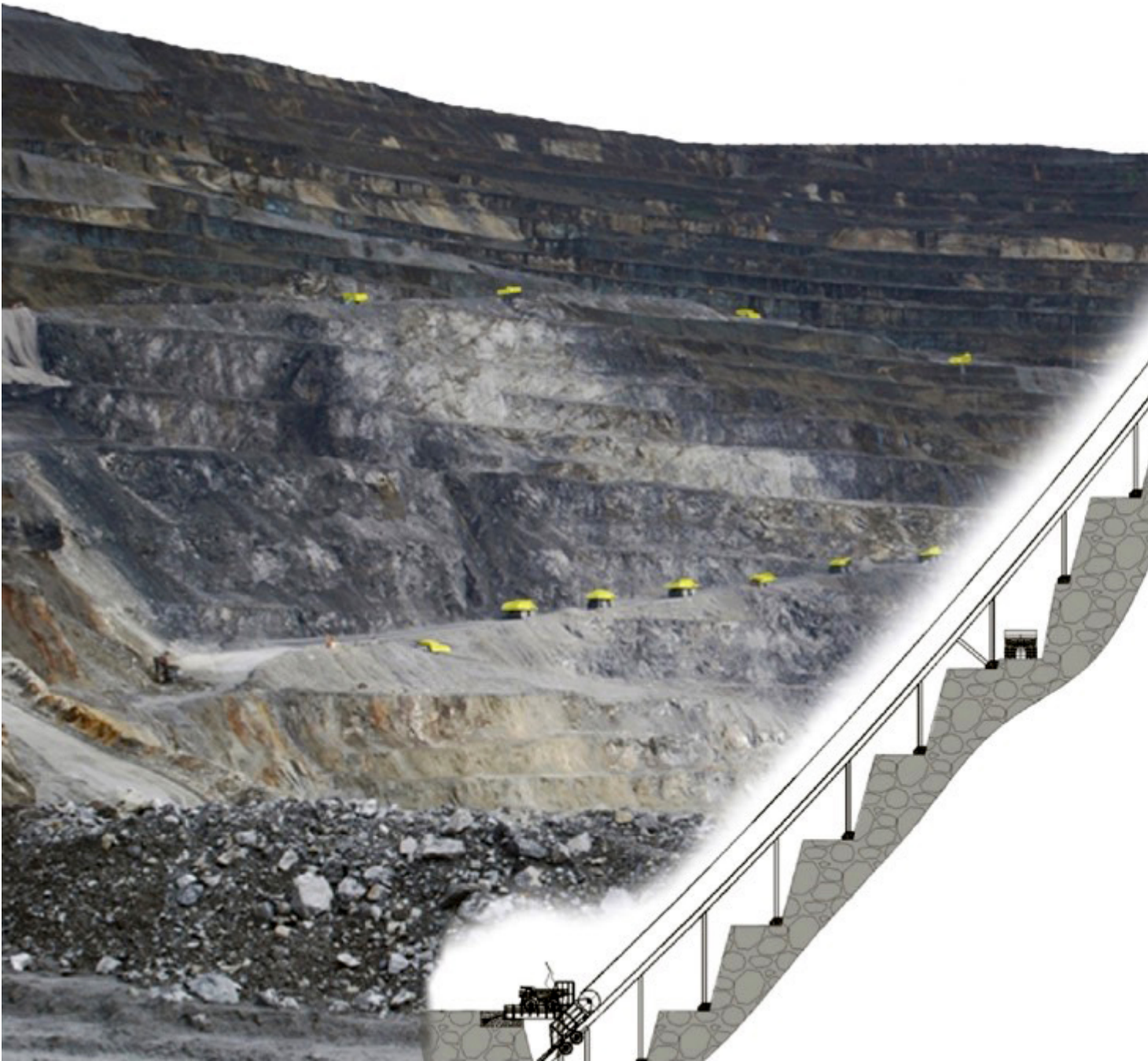
Fig. 4: Skip Conveyor System
