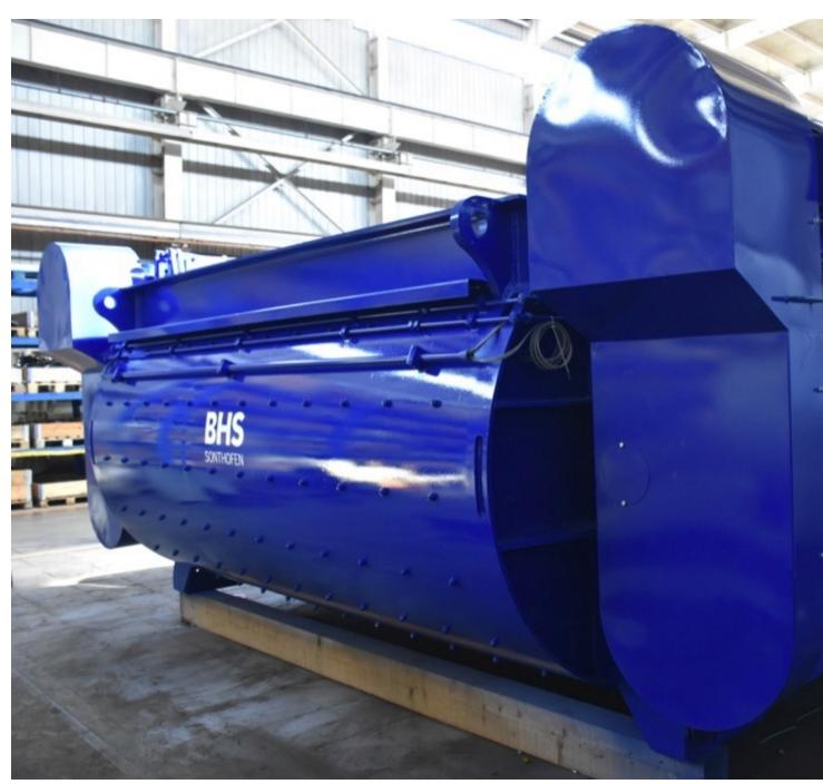
Twin-shaft batch mixers meet the highest demands for mixing
