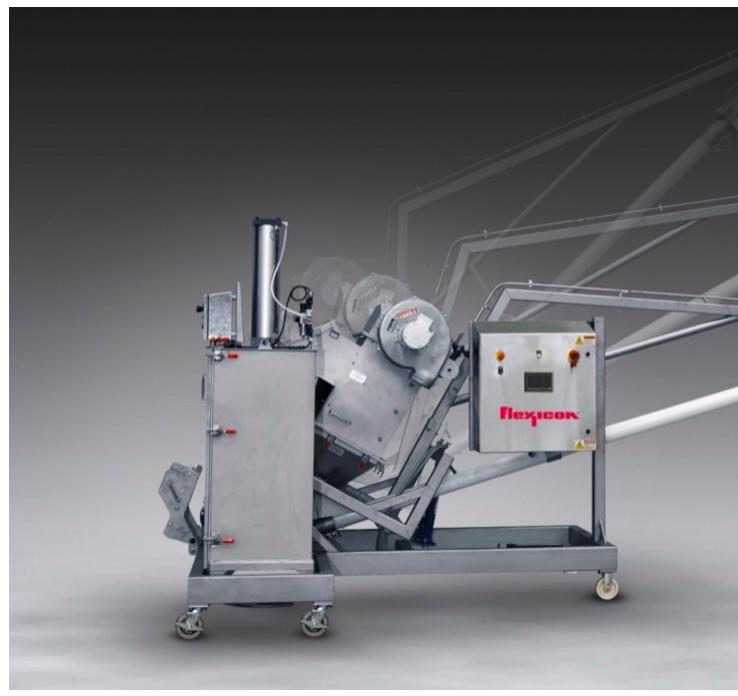
Flexicon Mobile Tilt-Down Flexible Screw Conveyor with Integral Bag Dump System can be deployed anywhere in the plant to transfer manually-dumped material into elevated process equipment, and compact empty bags, dust-free.
