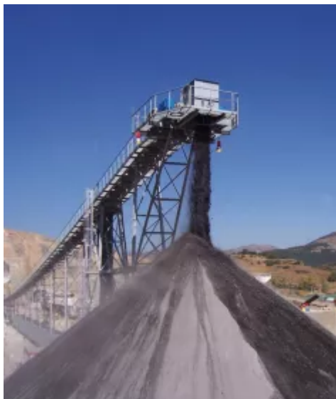
Fig. 1: Modular belt conveyor systems enable fast installation and dismantling and also increase reusability of components for temporary projects. (Picture: H+E Logistik GmbH)
