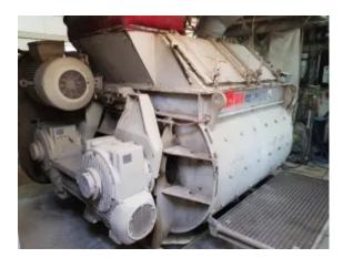
Maximum performance, even during continuous use: The twin-shaft batch mixer blends the complex formula in just 90 seconds.
