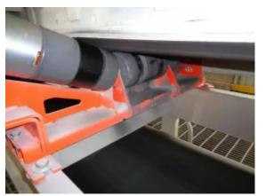
The load is carried by the generator's large support shaft, which is rigidly mounted to the idler support structure.
