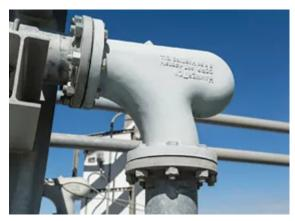
The teardrop-shaped vortex chamber designed into the curve of the Smart Elbow creates a deflection zone that minimizes elbow wear and product degradation without compromising material flow.
