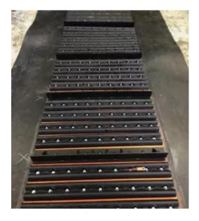
The solution: The 4B solution that was offered was to utilize 304 grade stainless steel fanged bolts, which have a significantly reduced magnetic resistance. This in turn almost completely eliminated the issues caused by standard mild steel bolts of being drawn to the fixed magnets. Which would cause excessive wear and reduce effective service life considerably.
