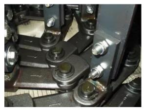
The Solution 4B offered its 4B142HAD heavy duty chain links with pins in AISI420 and circlips in AISI304.
