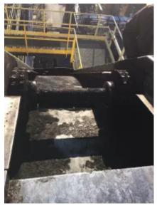
The chain conveyors where transporting a by-product of crude oil processing and were wearing extremely fast.
