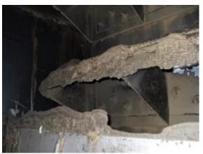
Oil and dust sticking to the traditional fabricated steel elevator buckets.
