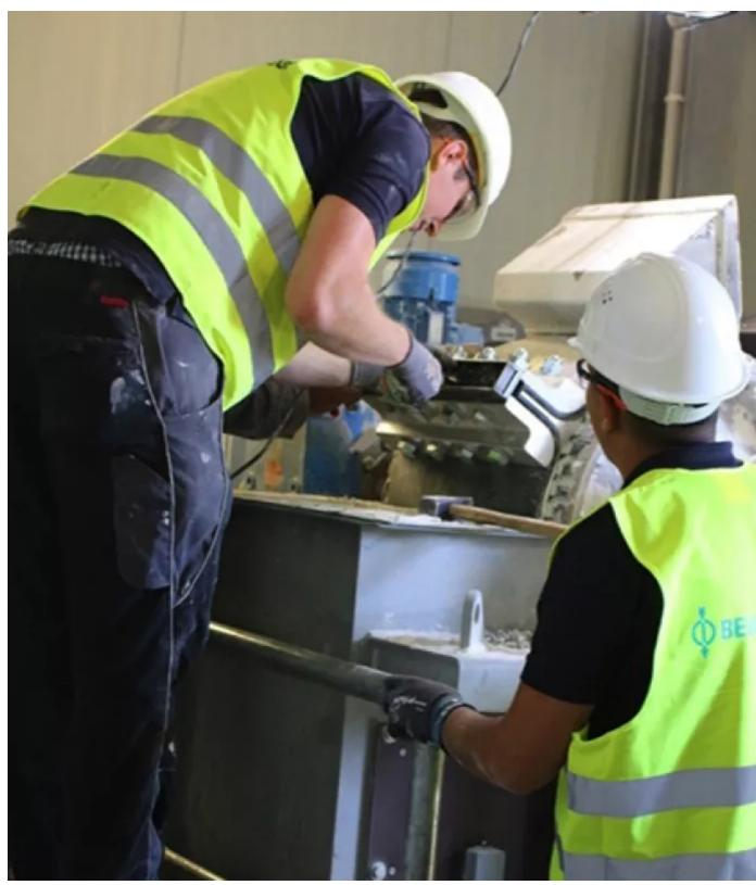
The ends of the steel cords are divided into individual strands in the U-shaped part of connection, twisted and cast with white metal.
