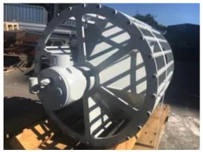
To avoid caking, the take-up pulley is designed as cage-type foot pulley and is provided with a double deflection cone. For this order, the screwed and hardened version of the cage-type foot pulley has been used.
