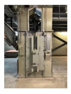
The parallel take-up device ensures that the take-up pulley is limited to parallel movement.
