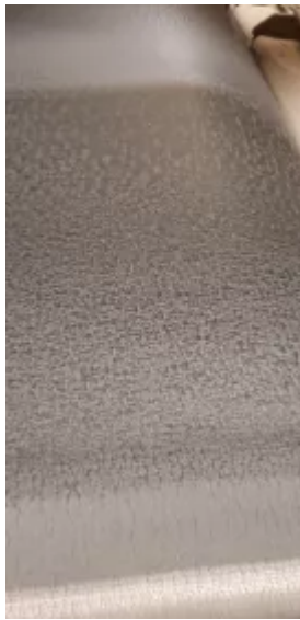
Close up of ozone cracked belt.
